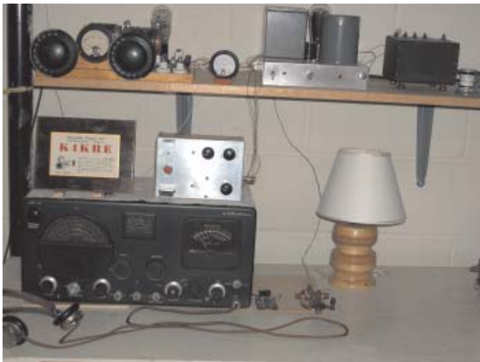
Second Station - Top Shelf - 80 Meter UX-210 Hartley 1929 Transmitter, Plate Current Meter, 300 Volt Power Supply, Antique Multitap Filament Transformer, Mid Level - 9 Watt 80/40 Meter 6AG7 Xtal Oscillator Transmitter, Table Level - Hallicrafters S-76 Receiver, Antenna Changeover Switch, Bunnell Straight Key
