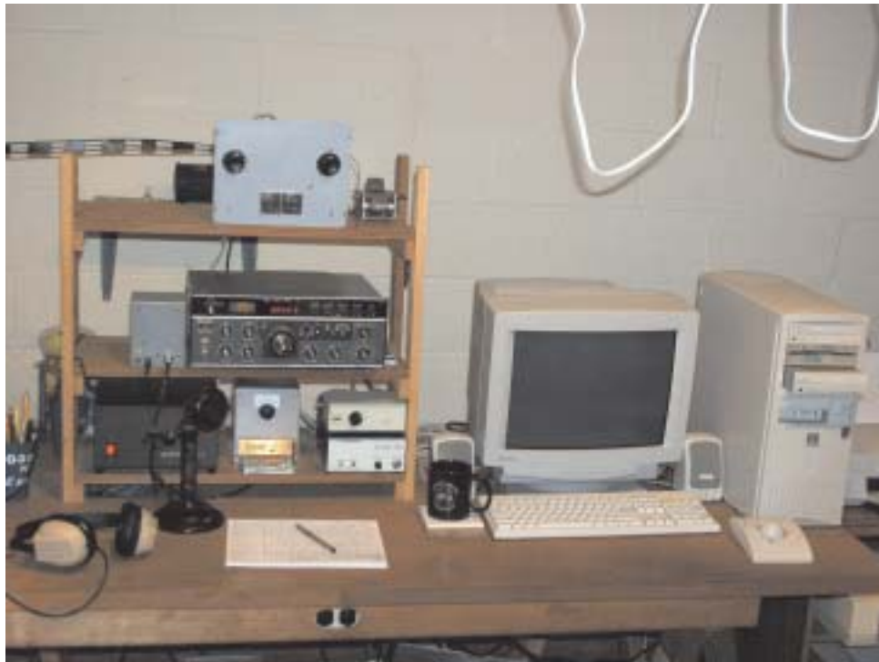
Top Shelf - Antenna Coupler - Ant: 90 ft cntr fed 450 line, Middle Shelf - Microphone Preamp / Slow Scan TV Filter, Ten-Tec Corsair Transceiver, Bottom Shelf - Power Supply, Front - Digital Clock, Rear - SSTV Mode Selector, Top Computer Parallel Port Select Switch, Bottom - View Port SSTV Adapter
